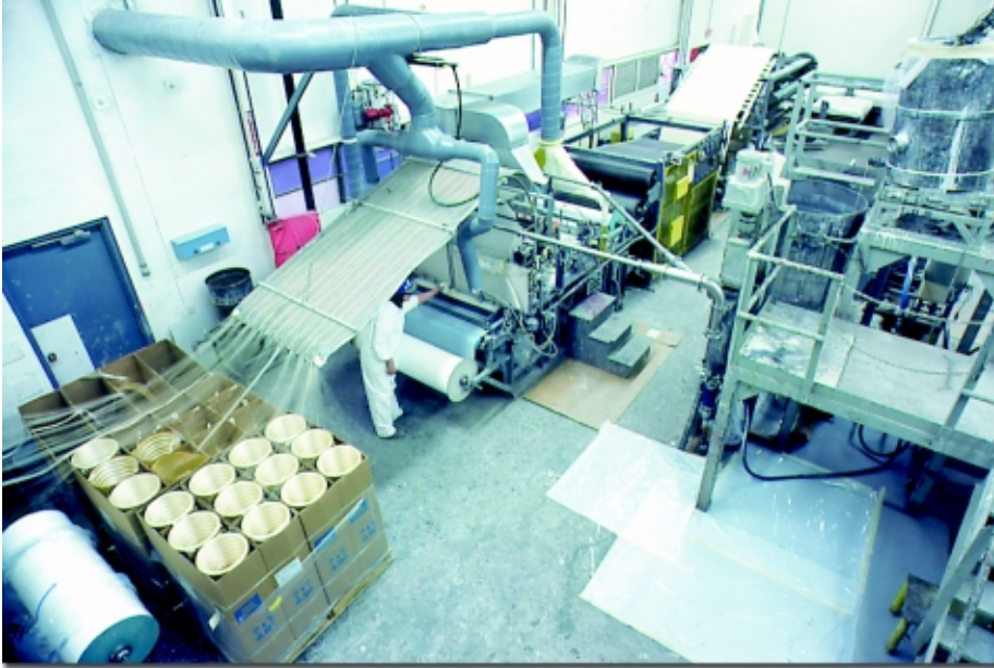
A continuous process creates a "sandwich" of glass and resin paste between sheets of film in SMC production.
