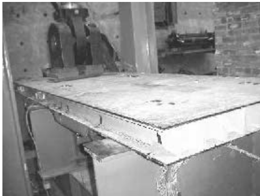
Fig. 54 Full-scale destructive tests on all-composite hybrid deck system for the Schuyler Heim Bridge, Long Beach, California. (Courtesy of University of California, Irvine, and California State University, Fullerton)
