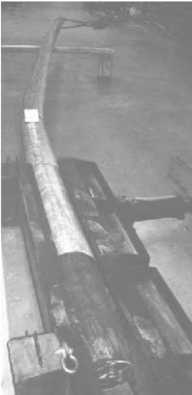
Fig. 14 Structural strengthening of utility wooden poles using polymer composites. (Courtesy of Fyfe Co. LLC)
