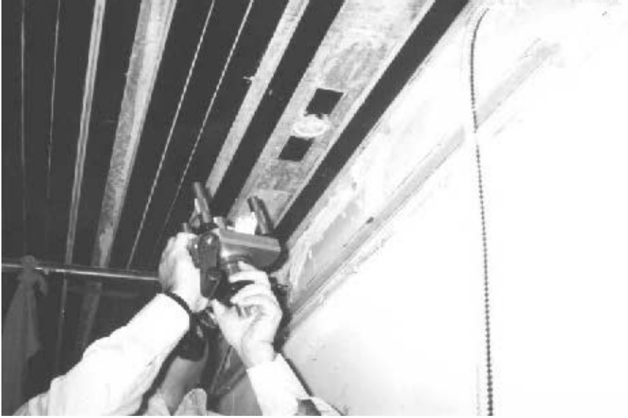
Fig. 22 Prefabricated composite laminate R/C slab applications and on-site bondline strength test. [Courtesy of Structural Composites Construction Inc. (SCCI)]
