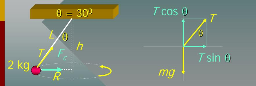
m = 2 kg; v = 5.32 m/s; R = 5 m; T = 22.6 N $F_c = \frac{mv^2}{R} \text{ or } F_c = T \sin 30^0 \qquad F_c = 11.3 \text{ N}$
