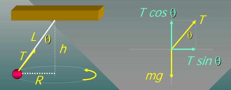
Note: The inward component of tension T sin θ gives the needed central force.
