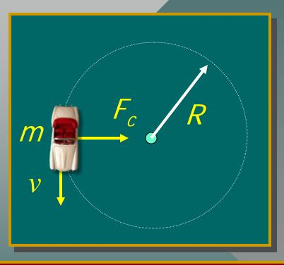
The centripetal force  $F_c$  is that of static friction  $f_s$ :
