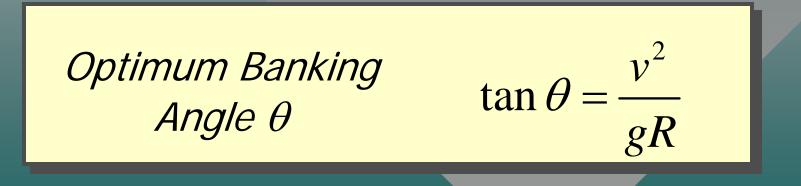
Example 5: A car negotiates a turn of radius 80 m. What is the optimum banking angle for this curve if the speed is to be equal to 12 m/s?
