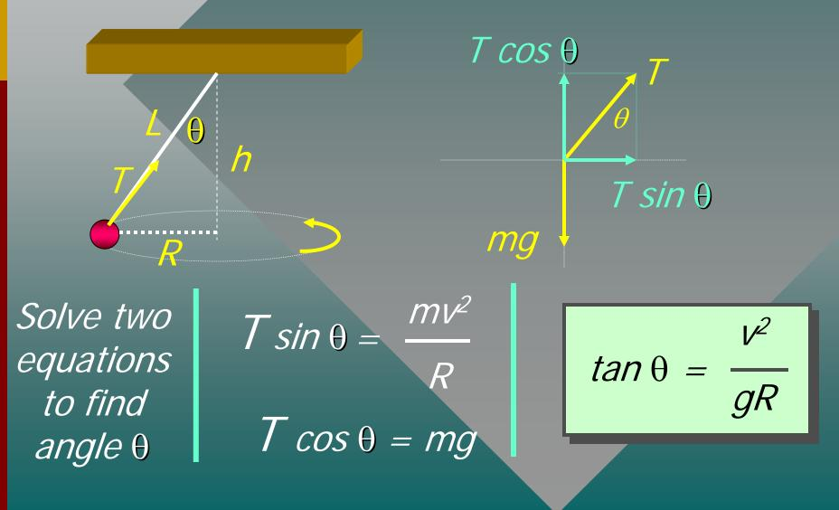
Example 6: A 2-kg mass swings in a horizontal circle at the end of a cord of length 10 m. What is the constant speed of the mass if the rope makes an angle of 30° with the vertical?
