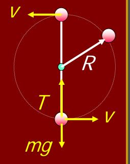
At Bottom:  $T - mg = \frac{mv^2}{m}$ R $T = \frac{mv^2}{m} + mg$ R $=\frac{(2 \text{ kg})(10 \text{ m/s})^2}{8 \text{ m}} + 2 \text{ kg}(9.8 \text{ m/s}^2)$ *T* = T = 44.6 NT = 25 N + 19.6 N
