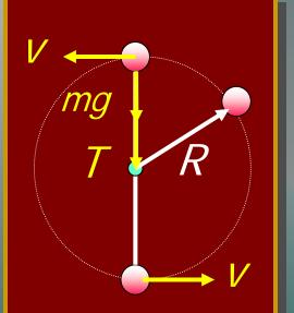
$\frac{mv^2}{At \ Top: \ mg + T = ---$ R $T = \frac{mv^2}{R} - mg$  $T = \frac{(2 \text{ kg})(10 \text{ m/s})^2}{8 \text{ m}} + 2 \text{ kg}(9.8 \text{ m/s}^2)$ T = 25 N - 19.6 NT = 5.40 N
