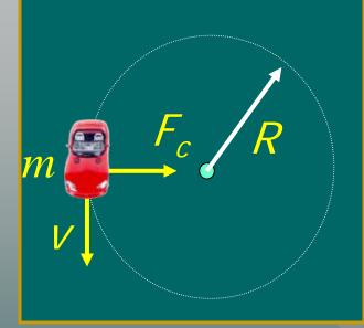
By banking a curve at the optimum angle, the normal force *n* can provide the necessary centripetal force without the need for a friction force.
