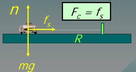
The central force  $F_c$  and the friction force  $f_s$ are not two different forces that are equal. There is just one force on the car. The nature of this central force is static friction.
