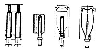
Injection stretch-blow moulding process sequence. a) Multiple injection moulding of preform b) Reheating stage c) Axial extension with telescopic mandrel (d) Blow moulding
