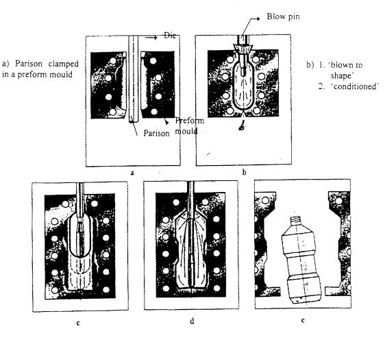
c&d) stretched to shape by an extension of the blow pin and by 'blowing air'.
