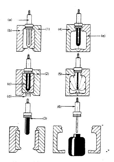
Injection blow moulding. 1, injection mould (b) containing transferable blowstick (a); 2. material injection via hot nozzle or runner (d) to form molten parison (c); 3. mould opens - blowstick removed with hot parison; 4, blowstick placed in blowing cavit (e); 5, air blown through holes in blowstick inflates parison; 6, blowing cavity opens - moulding removed.
